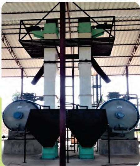
Digester with hatchery waste loading
