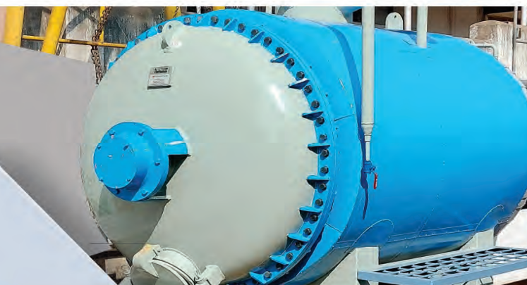
Digester (Cooker-Homogeniser-Vacuum Dryer)
