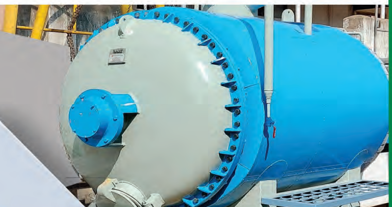
Digester (Cooker-Homogeniser-Vacuum Dryer)
